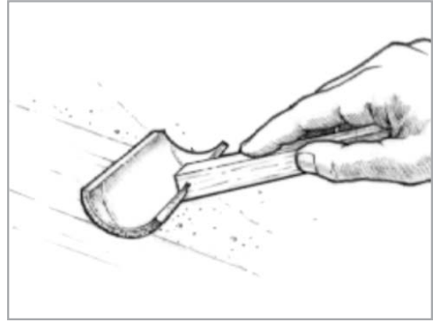
Figure 7-4 Tip off the coating by dragging a foam roller brush lightly over the fresh epoxy.
