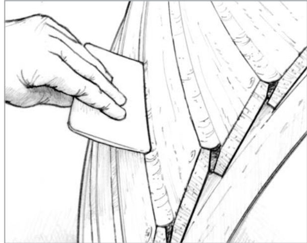
Figure 5-9 Fill the wet-out seam with thickened epoxy
