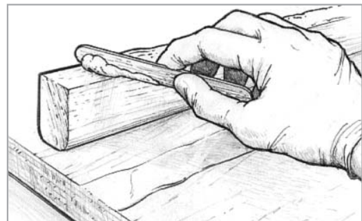
Figure 8-9 Apply thickened epoxy to one of the bonding surfaces.
