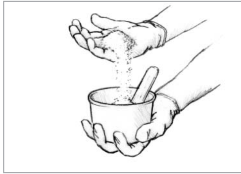
Figure 8-7 Blend in small handfuls or scoops of the appropriate filler until the desired consistency is reached.
