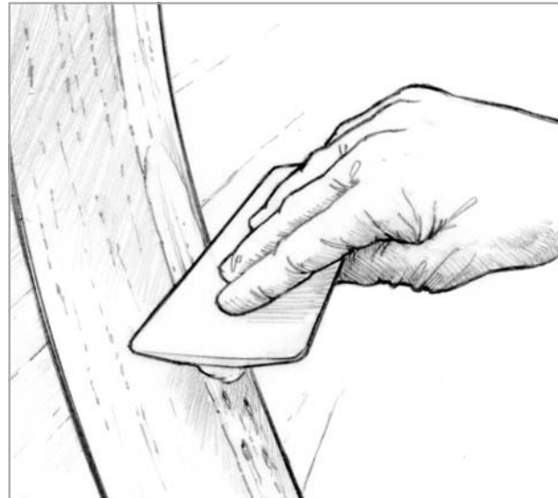
Figure 3-5 Fill the remaining voids with fairing compound.
