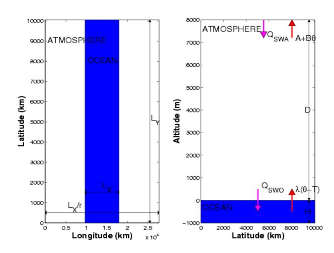
The domain geometry consists in one hemisphere with a single rectangular basin which dimensions are approximately the ones of the North Pacific. The only external forcing is the prescribed incoming solar radiation at the top of the atmosphere  $Q_{SWA}$  and at the ocean surface  $Q_{SWA}$ .
