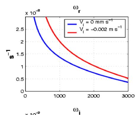
Note that the propagation term of baroclinic Rossby waves does not appear in the zonal mean equivalent barotropic vorticity equation, and yet a positive growth rate with a southward propagation appears. This figure shows that the mean current  $V_i$  does not modify significantly the growth rate and the southward propagation of the solution.
